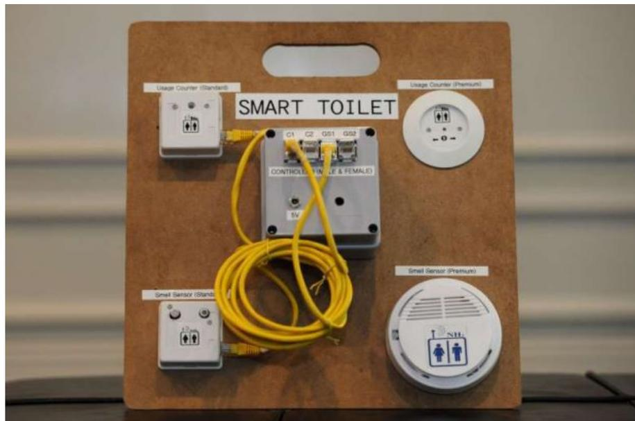
he Restroom Visitizer System (above) tracks how heavily toilets are used, and has a sensor to measure the odour levels of things like ammonia and hydrogen sulphide. The information is then sent to a portal that can be accessed through laptops and smartphones. - The Straits Times/Asia News Network
